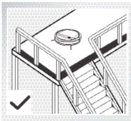
If there is a step or stairs in the cleaning area, please operate DEEBOT to ensure its Anti-Drop Sensors can detect the drop off. It may be necessary to place a physical barrier at the edge of the drop off to keep the unit from falling over the edge.
