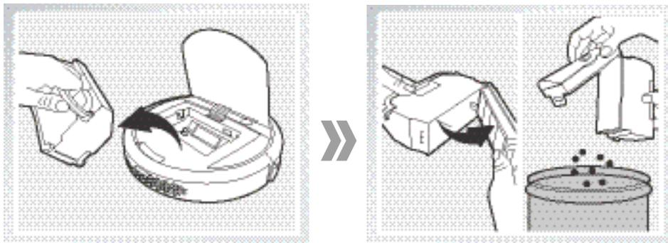
Remove the filters. Pat the High Efficiency Filter clean. Do not rinse the High Efficiency Filter under water.
